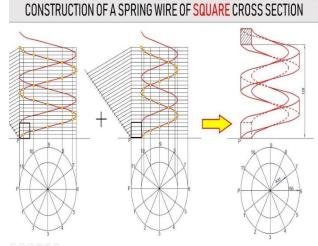
Given the centre line and starting point of a square helical spring, construct a left hand helical spring having the pitch of 60mm for 1 and half revolution.
